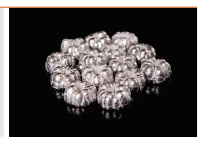
Nikkelverk NICKEL is guaranteed to meet the chemical requirements of ISO 6283 grade R9990 and ASTM B39-79.
